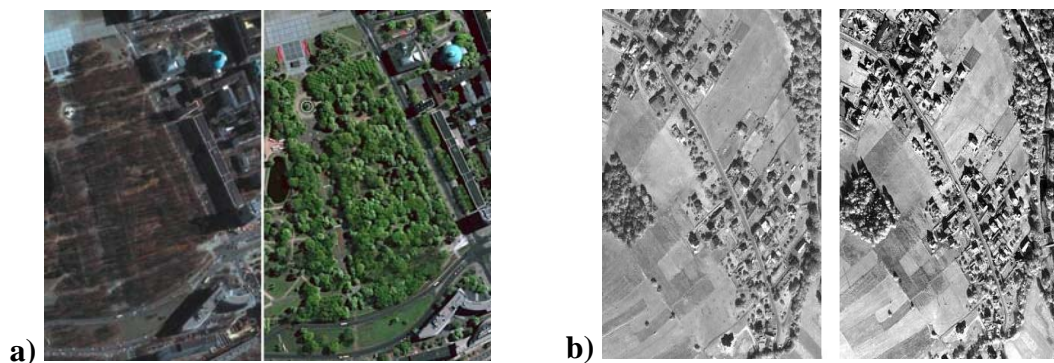
Figure 3. Four parts of VHRS imageries: Test field WAR (a): IKONOS (left), QuickBird (right); Test field NOTAR (b): IKONOS (left), QuickBird (right)
